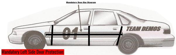
9 foot maximum C CHANNEL along the left drivers side (not to exceed 9 feet)  $1-\frac{1}{2}$  inch x 4 inch x  $1-\frac{1}{2}$  inch not to exceed  $\frac{1}{4}$  inch thick. Post to Post minimum.
